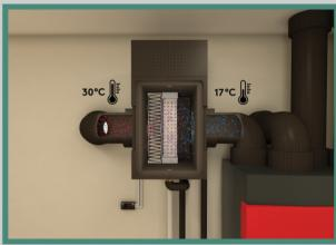
Geothermal energy generator uses ground coolness, that has a temperature of  $+10^{\circ}$ C to  $+14^{\circ}$ C in a 1,5m to 2,5m depth of the ground, ensuring cooling of the incoming air.
